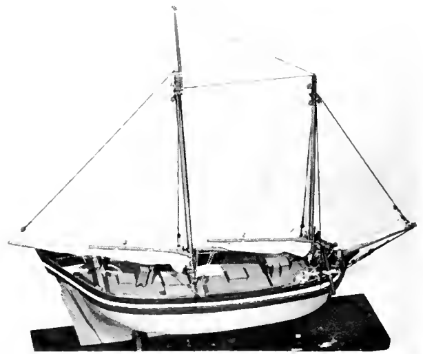
NEW ENGLAND PINKY of 1820-45, rigged model USNM 57586, showing a typical deck arrangement. The mainsheet horse forward of the tiller, however, is unusual and probably an error of the model builder. ( Smithsonian photo 44694. )
